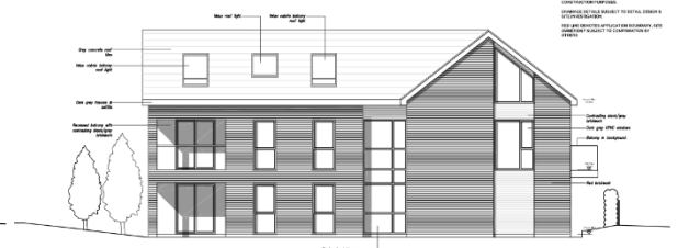
CHE/23/00313/FUL Revised south east and south west elevations showing amended ground floor window placement
